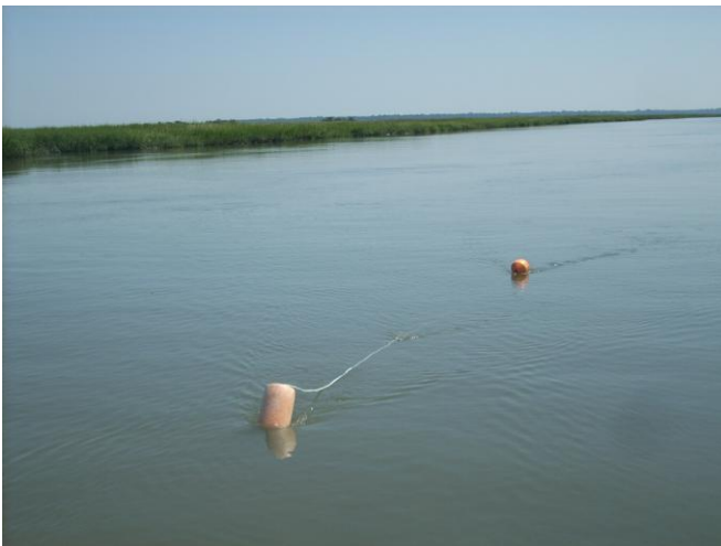
Figure 6. Second float visible from the surface and tag line Used to relocate the instrument at the end of the deployment period.
