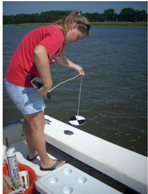
Figure 3. Measuring secchi depth at a water quality monitoring site.
