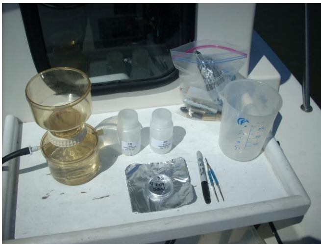
Figure 2. Filtration set up for TDN, TDP and chlorophyll a .
